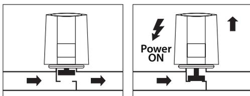
Function display for NO versions extends only when valve is fully closed by approx. 0.5 mm.
