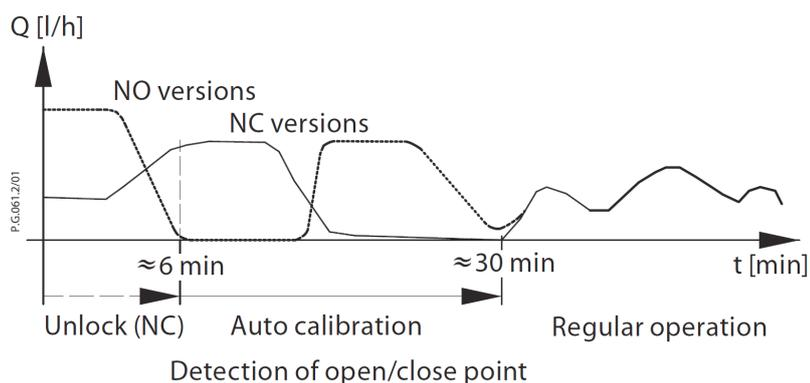
Automatic initial calibration procedure to actual preset AB-QM stroke (detection of opening and closing point). ABNM A5 actuator needs ~30 min. for first calibration (including First Open Function (NC versions only) and valve open and close point detection. In case of power loss the actuator will remember its position and will not need recalibration.
